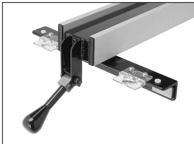
Figure 32. Fence knob installed.
